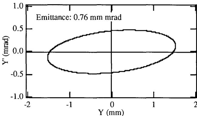
Figure 8: The beam ellipse in vertical phase space obtained by using the results of figure 6.
