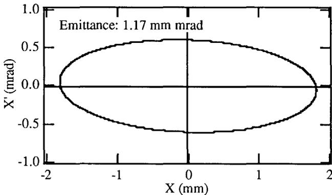
Figure 7: The beam ellipse in horizontal phase space. A result of the measurements in figure 5.
