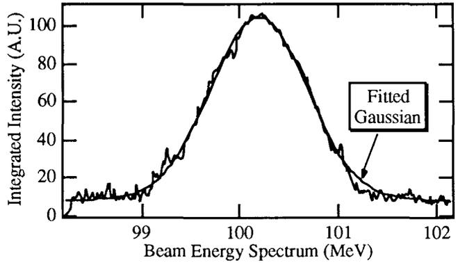
Figure 4: Energy spectrum of an optimised 150 ns pulse. Total charge in the pulse 3.45 nC. Also shown is a Gaussian function fitted to the data.
