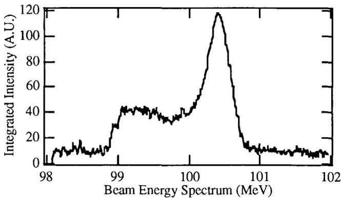
Figure 3: Energy spectrum for a long pulse 300 ns. Total charge in the pulse was 11.4 nC.
