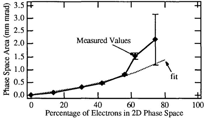
Figure 9: The diagram shows that approximately 60% the beam in two dimensional phase space can be considered to be distributed Normally. (The dotted line is the theoretical curve based on a Gaussian distribution normalised to the first four points. Multi-bunch mode 310 ns, 10 mA.)
