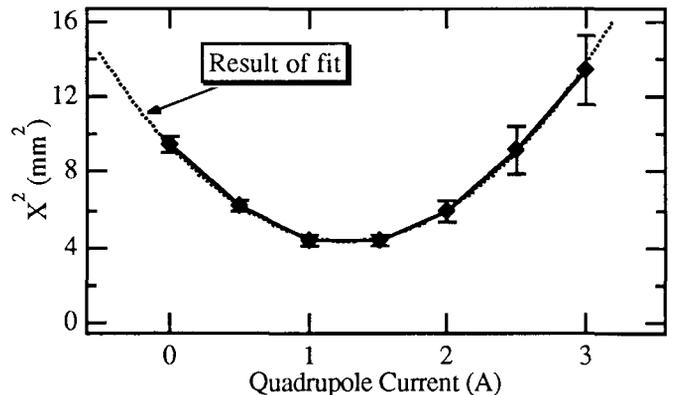
Figure 5: Variation of the square of the horizontal beam size as a function of quadrupole current.
