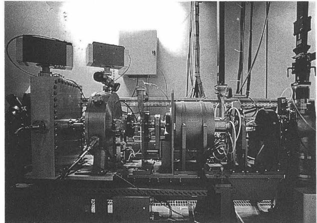
Figure 1. Gun and bunching sections.
