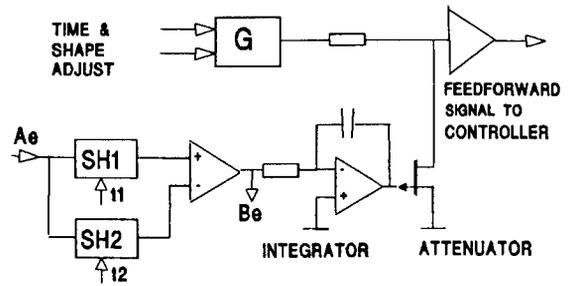
Figure 5: Simplified schematic of the simulated feedforward loop.
