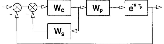
Figure 3: Illustration of the Smith controller.
