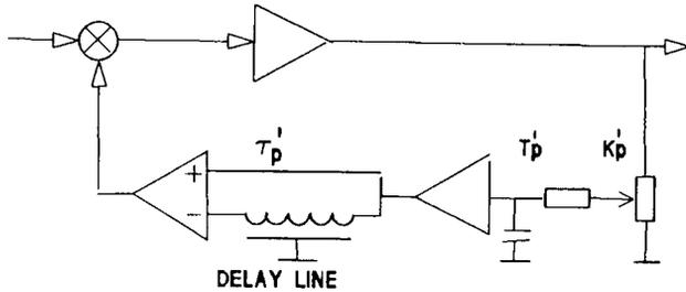
Figure 4: Simplified schematic of the Smith controller.
