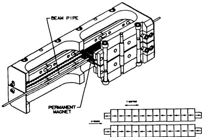
Fig. 3 Schematic of Advanced FEL permanent magnet wiggler.
