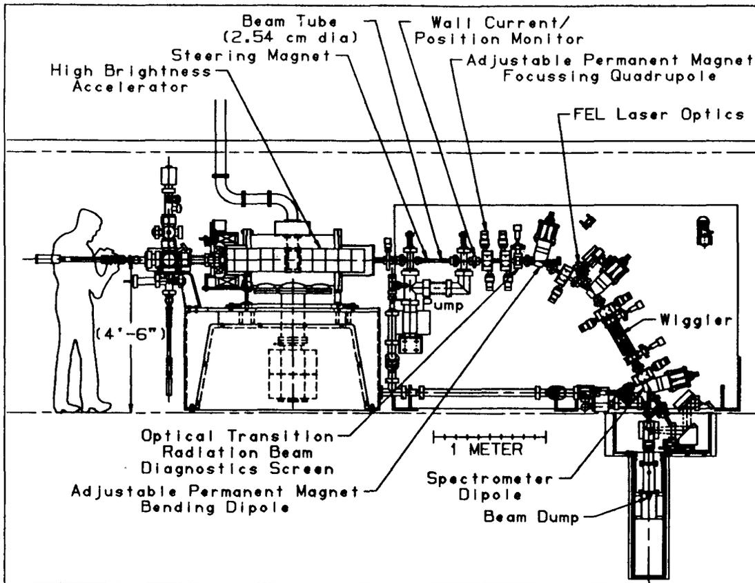
Fig. 1 Schematic of the Advanced Free-Electron Laser.
