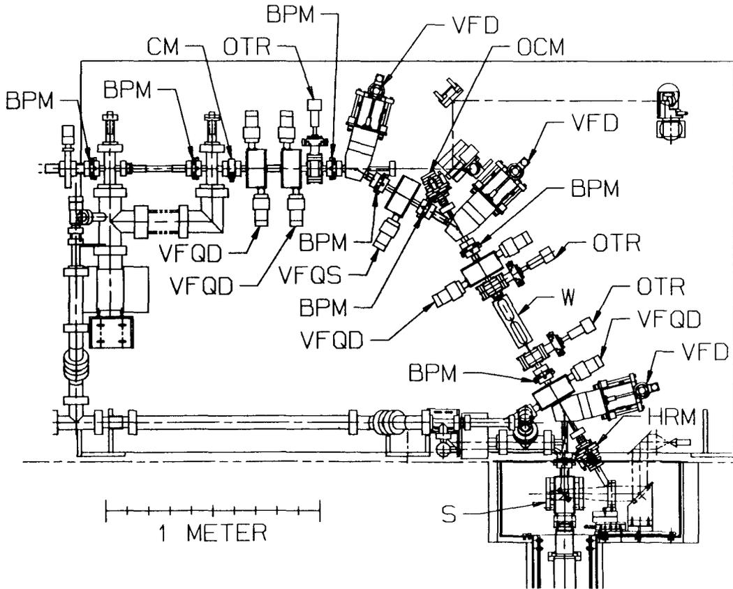
Fig. 2 Layout of the Advanced FEL beamline. BPM: Beam Position Monitor; CM: Current Monitor; HRM: High Reflectivity Mirror; OCM: Output Coupling Mirror; OTR: Optical Transition Radiation; VFQD: Variable Field Quadrupole Doublet; VFQS: Variable Field Quadrupole Singlet; VFD: Variable Field Dipole; S: Spectrometer; W: Wiggler.
