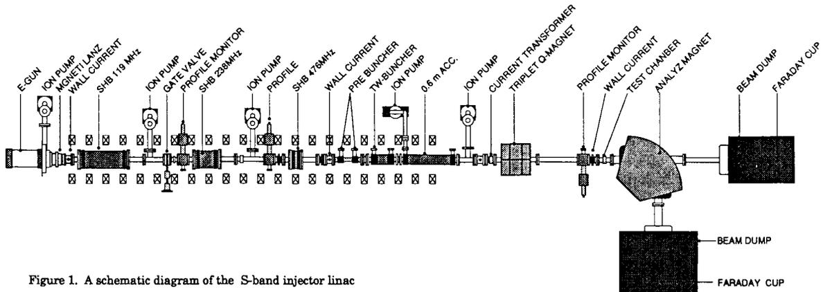
Figure 1. A schematic diagram of the S-band injector linac
