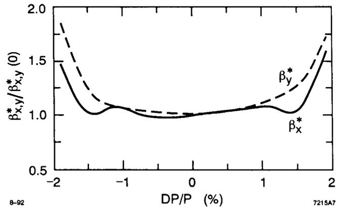
Fig. 5. Energy passband of the DLC Final Focus.
