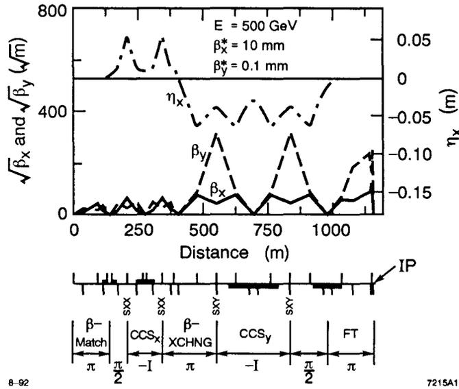
Fig. 1. Optics of a "Generic" Final Focus System.
