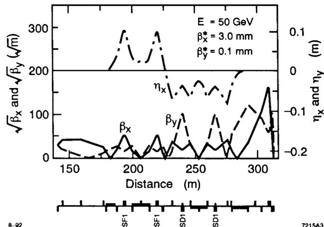
Fig. 3. Optics of the Final Focus Test Beam.
