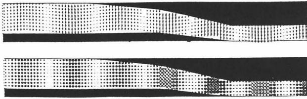
Fig. 8 Electric and Magnetic Fields of Travelling Wave at Steady State in X-Band Transducer.
