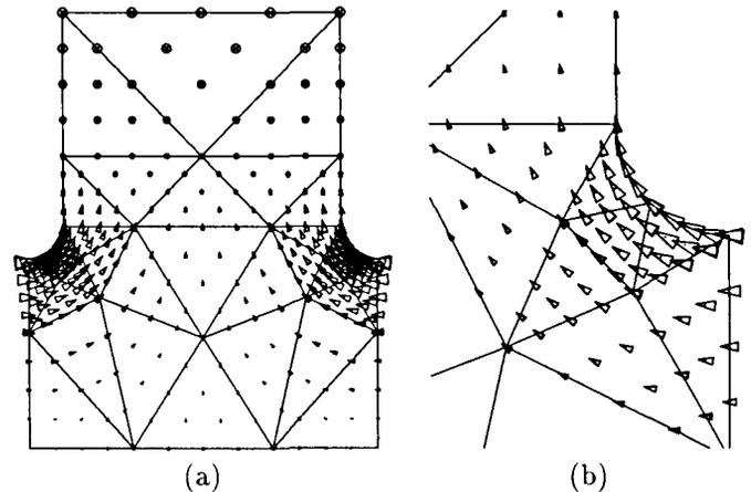
Fig. 4 (a) Lowest dipole  $\pi$  mode for an x-band accelerator structure and (b) magnified view of the right nose. The arrows represent the field  $(B_z, B_\rho)$  and the circles represent the field  $-i\rho B_\phi$ . The sizes of the circles and arrows indicate the magnitude of the fields.
