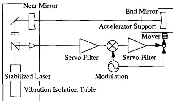
Fig. 4 Possible conceptual design of the transverse alignment.
