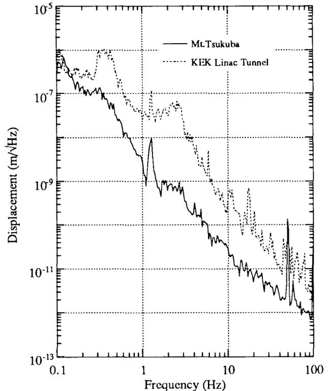
Fig. 3 Fourier spectrum density of vibration at Mt. Tsukuba and the KEK linac.
