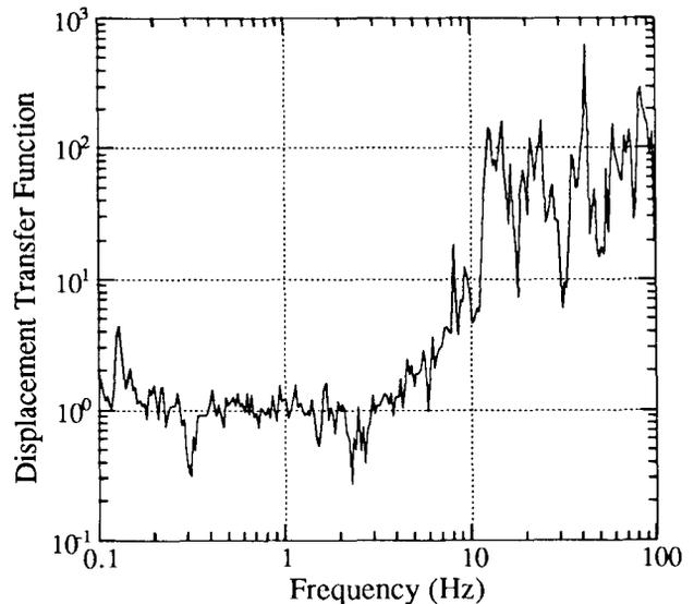
Fig. 5 Transfer function of the accelerator support to the ground.
