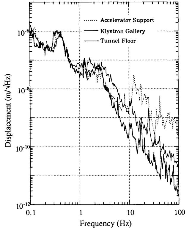
Fig. 2 Fourier spectrum density of vibration at the KEK linac.
