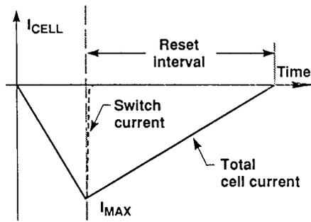
Figure 5b Idealized waveforms for the circuit in Figure 5a.
