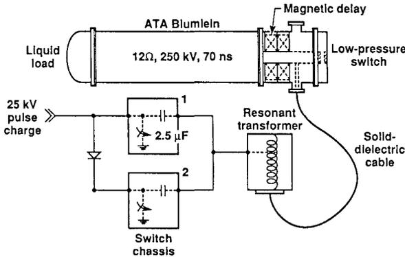
Figure 3 Circuit diagram of the two-pulse test apparatus for magnetically-delayed low-pressure switch experiments.
