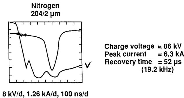
Figure 4 Voltage and current waveforms for a low-pressure switch closure in nitrogen. Electrodes are flat with a stainless-steel anode and aluminum cathode. N<sub>2</sub> flows into the gap region via an axial trigger electrode. Gas pressure in the cathode trigger plenum is 204 μm while the pressure at the chamber wall measures 2 μm. Radial pressure distribution in the 1-cm gap region is unknown.
