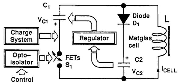
Figure 5a Circuit architecture for the proposed ILSE recirculator.
