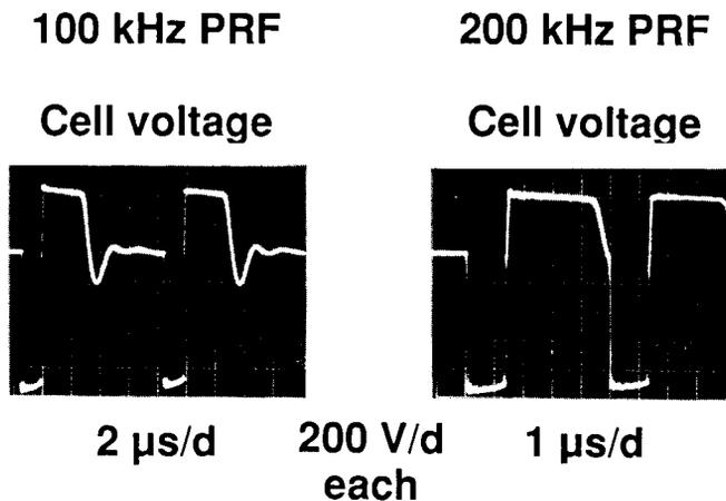
Figure 6 Two-pulse test of the modulator circuit with a small FET array. Voltages shown are measured across the Metglas induction core for a 100-kHz and a 200-kHz repetition rate.
