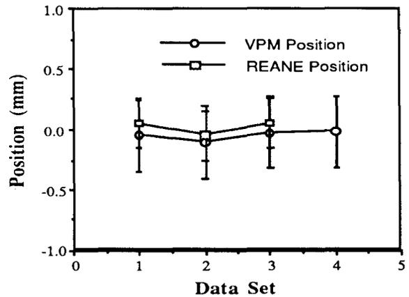
Fig. 6. Vertical beam centroid location as measured using the slit and collector gear and the VPM for several IMS output quad settings.
