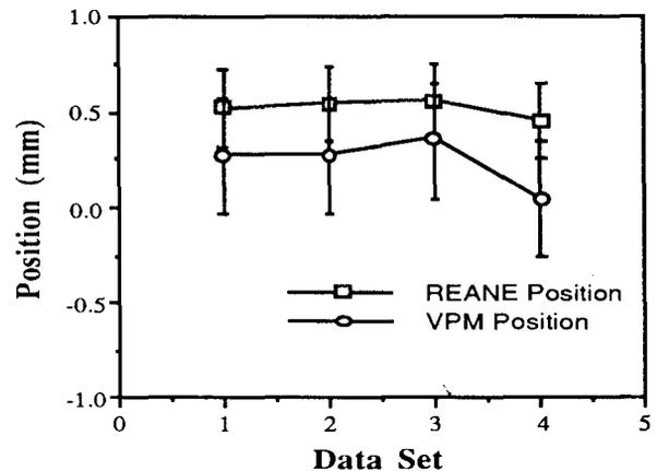
Fig. 7. Horizontal beam centroid location as measured using the slit and collector gear and the VPM for several IMS output quad settings.
