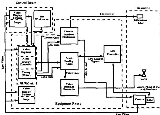
Fig. 2. Video profile diagnostic block diagram.
