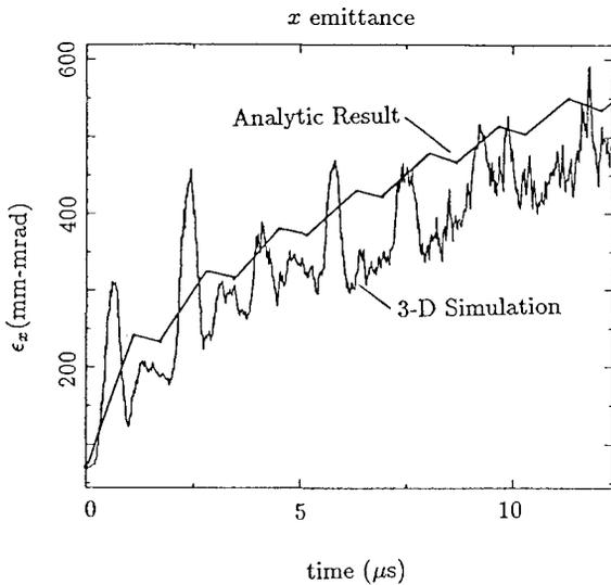
Fig. 1. Emittance growth in a racetrack. The parameters are  $\sigma_0 = 72^\circ$ ,  $\sigma = 8^\circ$ ,  $\rho = 3.6\text{m}$ ,  $Am_p \beta^2 c^2 / 2 = 10\text{MeV}$ .
