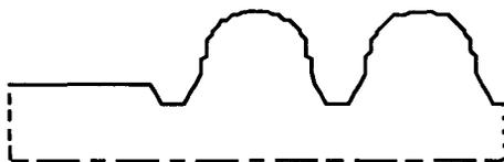
Fig. 3. End tube and first two cells for the case with a nose on the end tube.
