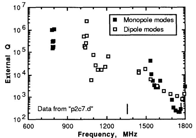
Fig. 6. External Q's for the p2 cavity, which is similar to the TESLA LTP cavity, but for a beta of 0.9759.
