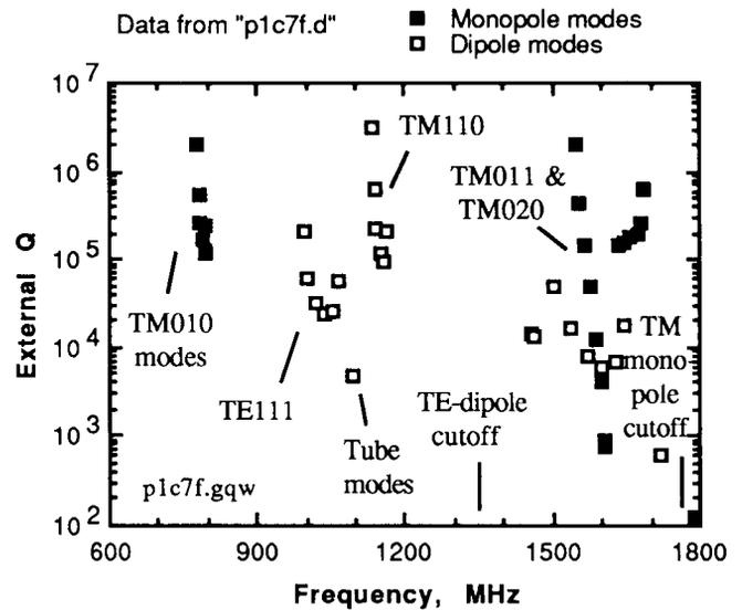
Fig. 1. Characterization of the higher-order modes of the PILAC cavity. The resistive band was 78.7 mm wide, beginning 12.1 mm away from the end cell.
