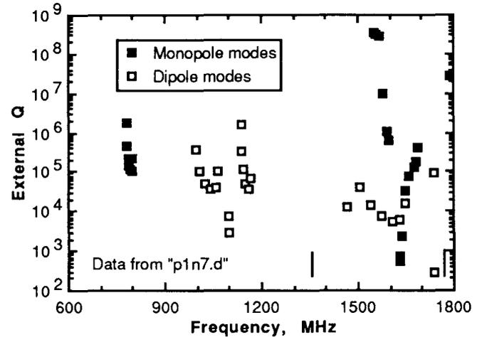
Fig. 5. Effect of width of end cells: End cells narrower than mid cells by 6.057 mm.
