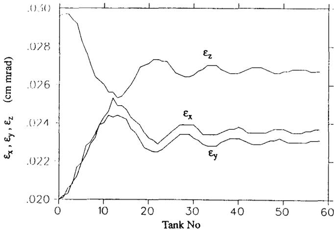
Figure 2: Normalized rms transverse ( $\epsilon_x, \epsilon_y$ ) and longitudinal ( $\epsilon_z$ ) emittances as function of tank numbers.
