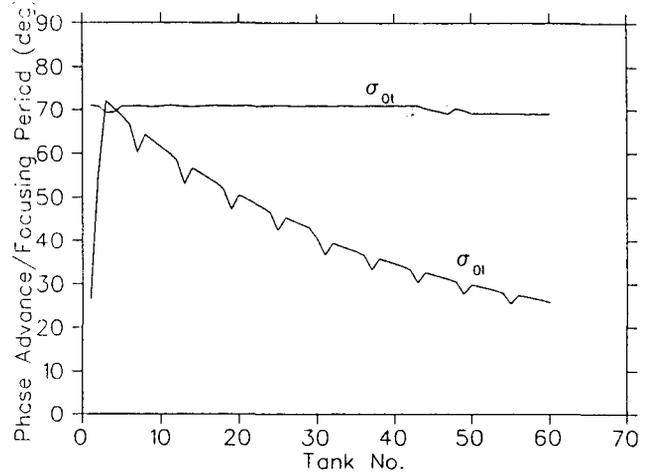
Figure 1: Zero-current transverse and longitudinal phase advances in the CCL as function of tank numbers.
