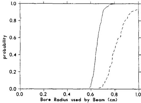
Figure 4: Probability distribution of the bore radius used by the beam for a combination of random errors given in Table 3. Graph shows the probability that the beam radius will be at or below the plotted value.
