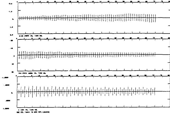
Figure 3: Beam size, phase and energy profiles as the beam traverses the CCL.
