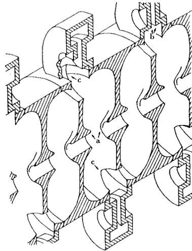
Fig. 2. Spark locations: a) accelerating-cell nose cones, b) coupling-cell nose cones, c) coupling slots.
