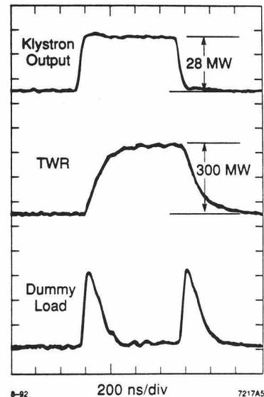
Figure 2. TWR Waveforms
