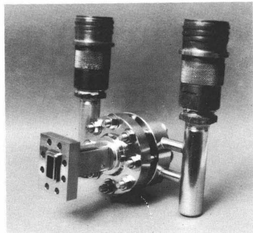
Figure 5. 50 MW Grapefruit Load bakeable to 550°C
