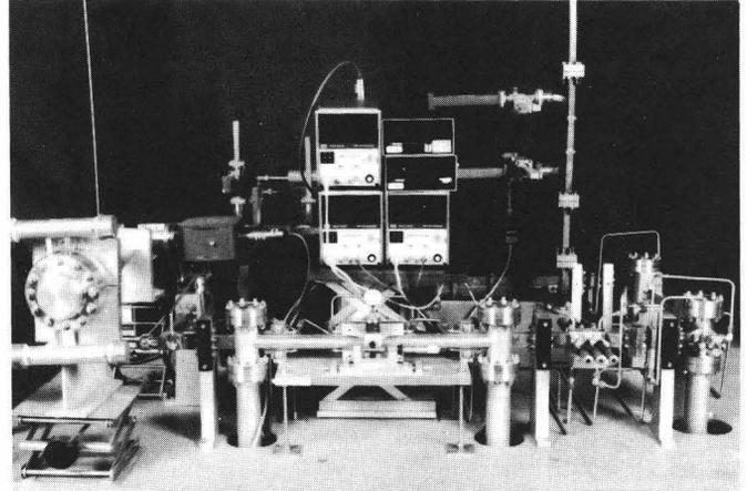
Figure 1. X-band Traveling Wave Resonator
