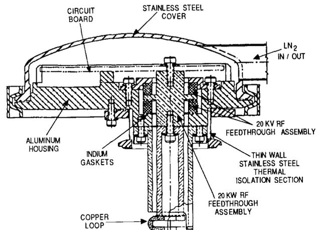
Fig. 2. The fast-tuner unit, which operates at 77 K. The copper loop projects into the superconducting cavity, and can couple as much as 30 KVA of reactive power into the tuner. The overall diameter is approximately six inches.
