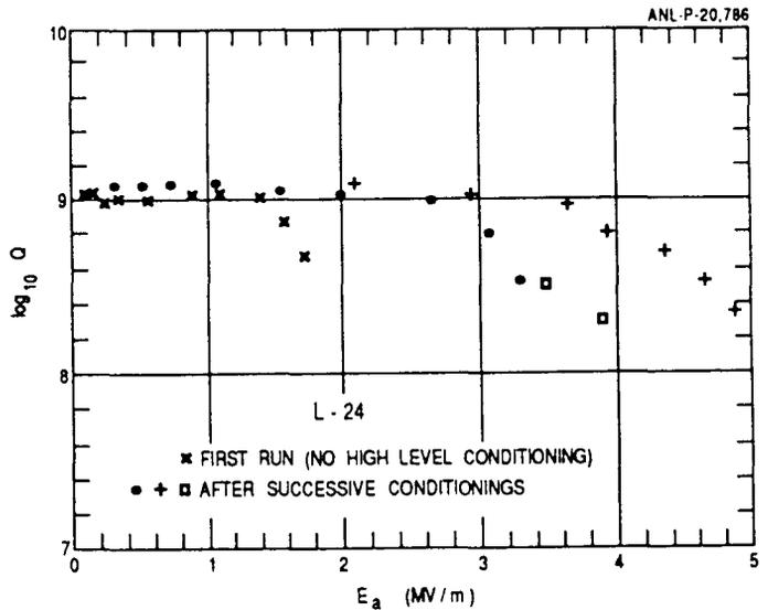
Fig. 3 Q curve against average electric field for L-24
