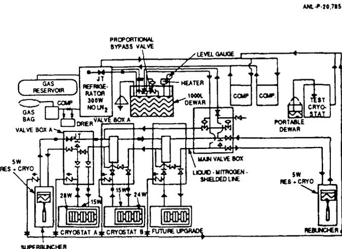
Fig. 2 Schematic view of the helium distribution system
