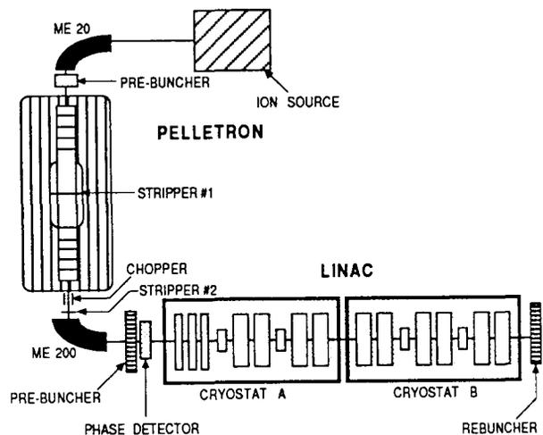
Fig. 1 Schematic view of the projected Pelletron-Linac System
