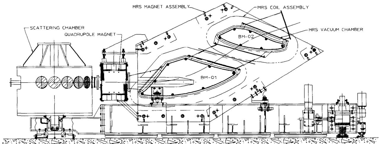
FIG. 1 LAMPF MEDIUM RESOLUTION SPECTROMETER (MRS) ASSEMBLY
