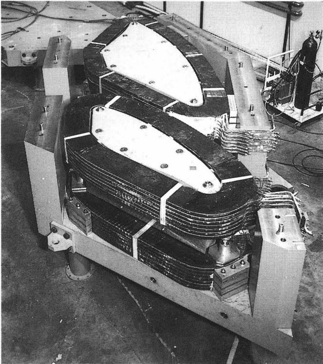
Fig. 4 MRS Magnet Assembly (One Yoke Removed)
