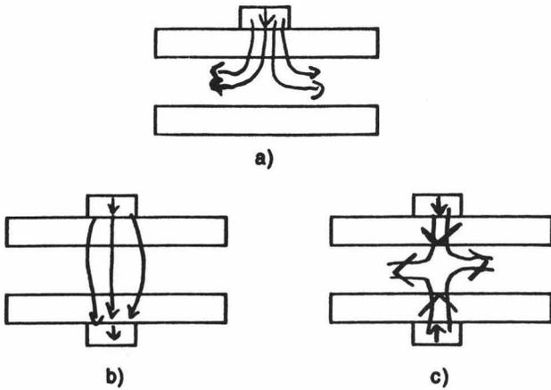
Fig. 1 (a) A single magnet used to correct vertical dipole (skewed quadrupole) causes a skewed quadrupole (vertical dipole) error; (b) a better way to correct a vertical dipole error; (c) a better way to correct a skewed quadrupole error.
