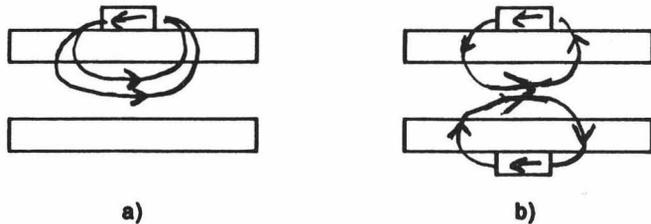
Fig. 2 (a) Correcting a  $B_x$  dipole error with a single horizontally polarized corrector, introducing a normal quadrupole error; (b) a better way to correct the dipole error.
