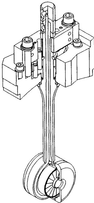
Fig. 2 Drift tube and mounting.
