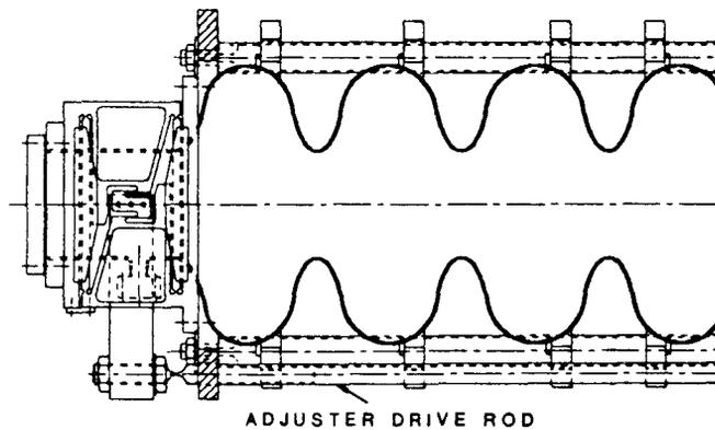
Fig. 2. Adjuster mechanism for end half-cell tuning.
