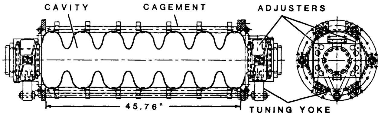
Fig. 1. Seven-cell 805-MHz cavity assembly.
