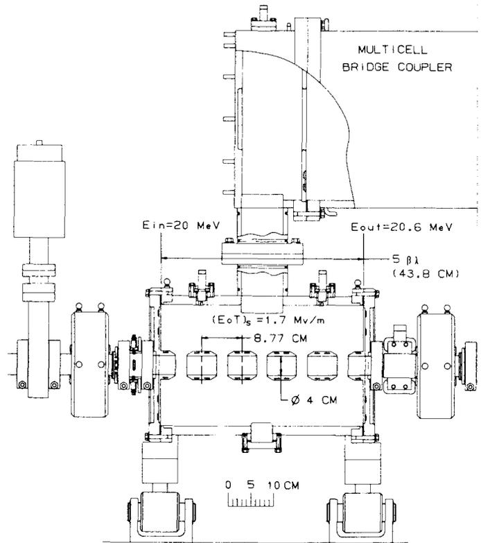
Fig. 3 Internal structure of the 20.6-MeV 700-MHz BCDTL accelerating tank ( $5 \beta\lambda$  long).
