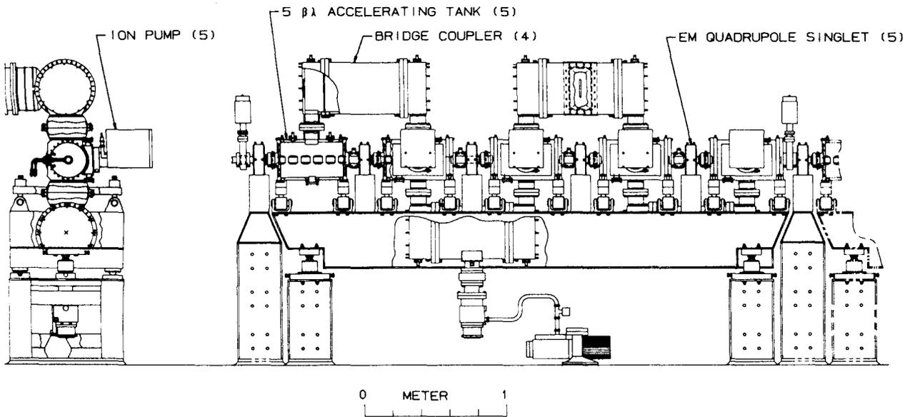
Fig. 2 5 tank 20-22.9 MeV, 700-MHz bridge-coupled DTL module.
