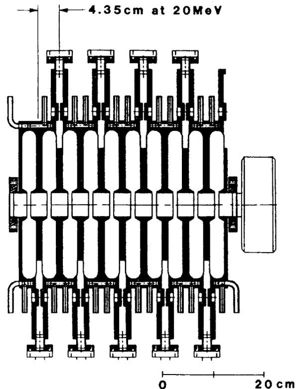
Fig. 1 A  $5\beta\lambda$  long CCL accelerator tank at 20 MeV and 700 MHz showing close end wall spacing and fabrication complexities.
