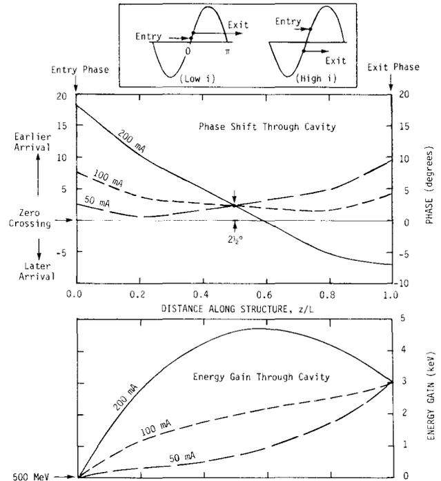
Fig. 2. RF Cavity Phase Shift and Energy Gain vs Distance Along Structure for  $P_0 = 8\text{kW}$  and  $V_0 = 500\text{MeV}$  (0.11%  $\Delta V/V$ ).
