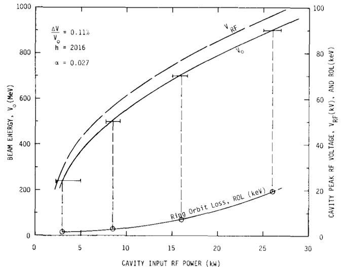
Figure 1. Traveling Wave Structure Input Power and Peak RF Voltage versus Beam Energy and Ring Orbit Loss.
