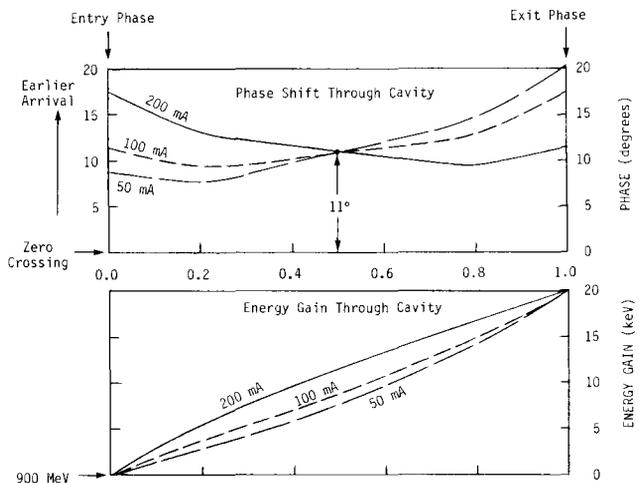
Fig. 3. RF Cavity Phase Orbit and Energy Gain vs Distance Along Structure for  $P_0 = 26\text{kW}$  and  $V_0 = 900\text{MeV}$  (0.11%  $\Delta V/V$ ).
