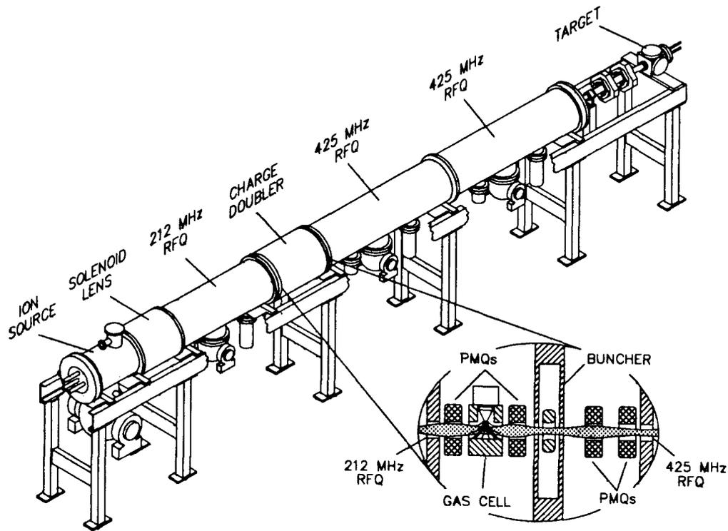
Figure 1. Line drawing of the SAIC PET Isotope Production Accelerator
