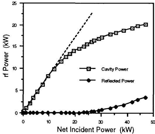
Fig. 5. GTA IMS Buncher B cavity and reflected-power response.
