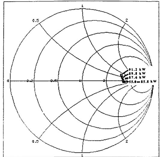
Fig. 3. RFQ impedance response after 30 hours of reconditioning.
