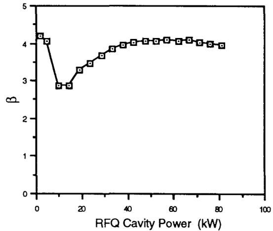
Fig. 4. GTA RFQ drive-line coupling as a function of cavity power.
