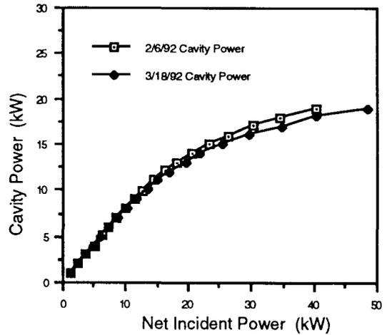
Fig. 8. GTA IMS buncher B cavity power response for two separate days.
