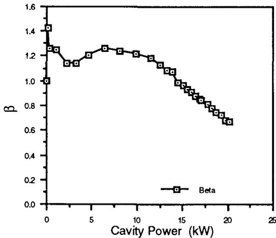
Fig. 6. GTA IMS Buncher B drive-line coupling ( $\beta$ ) power response.
