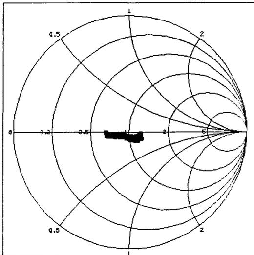
Fig. 7. IMS buncher B impedance from 0 to 20 Kilowatts.
