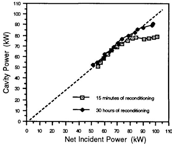
Fig. 1. GTA RFQ power response during reconditioning.
