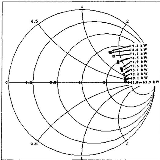
Fig. 2. RFQ impedance response after 15 minutes of reconditioning.
