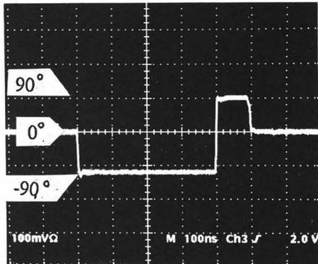
Fig. 5 Observed input pulse phase (low-level).
