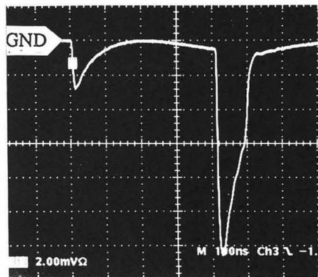
Fig. 6 Observed output of the SLED (low-level).
