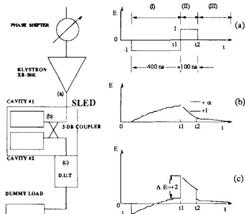
Fig. 1 Schematic diagram of high-power RF test-bench using the SLED. When the klystron output wave (a) is supplied, the emitted wave (b) from the cavity and compressed wave (c) transmitted to the device-under-test (D.U.T) appear as illustrated, respectively.
