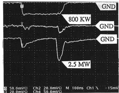
Fig. 7 Observed output signal of the SLED in the high - power test. Klystron output (top), reflected power to the klystron (middle) and output of the SLED (bottom) are shown.
