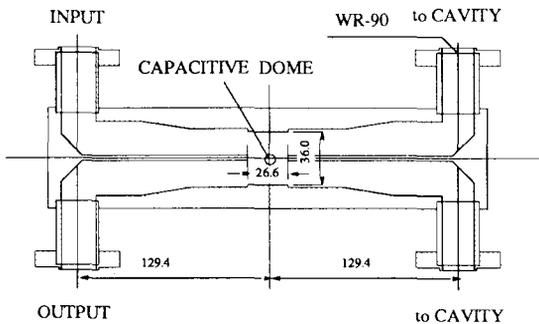
Fig. 2 Cross-section view of the 3-dB coupler.
