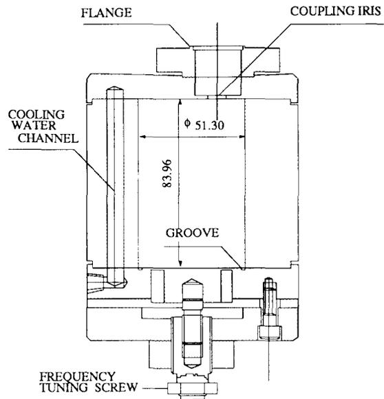
Fig. 3 Cross-section view of the cavity.
