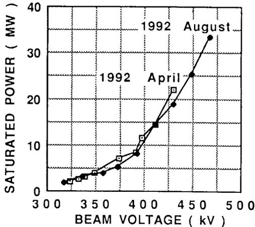
Fig-3) XB-72K perveance curve
