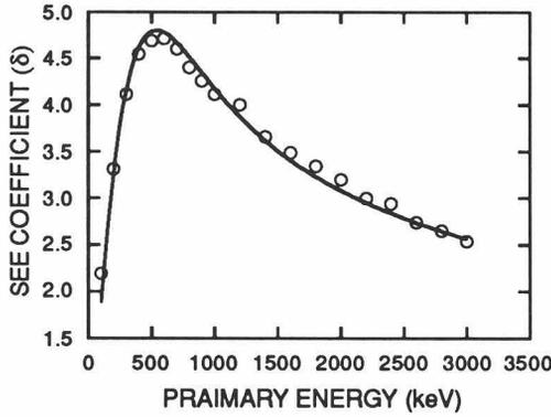
Fig. 2 Secondary electron emission (SEE) coefficient of an alumina as a function of primary energy. The open circle is the measured data by Dawson[10], and solid line is fitted with eq. (2)
