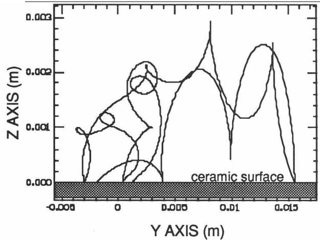
Fig. 3 The typical trajectory of the simulated multipactoring electron at the power of 4 MW.
