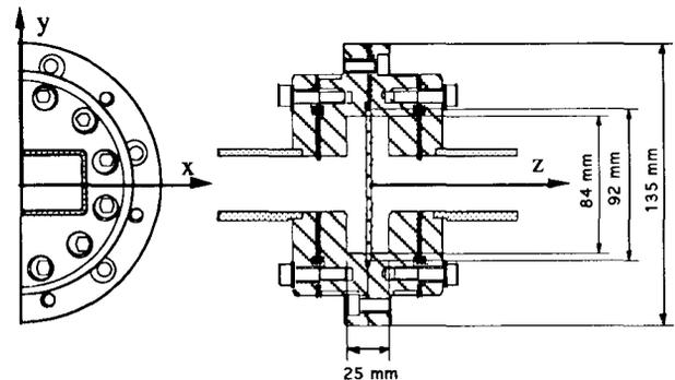
Fig. 1 The structure of the rf window
