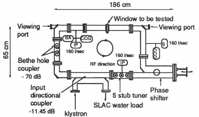
Figure 6 Schematic drawing of the resonant ring
