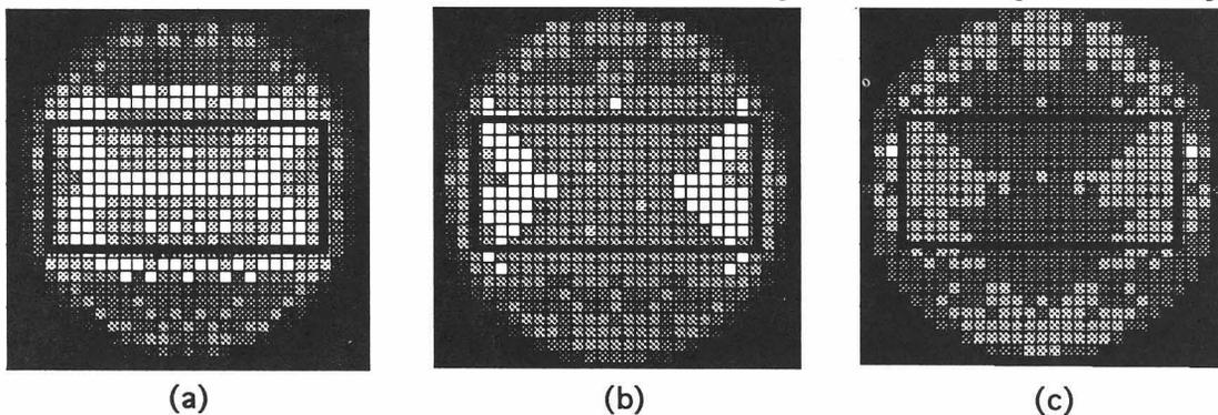
Fig. 4 The density distributions of number of impinging electrons at the power level of (a) 4 MW, (b) 10 MW and (c) 50 MW. The rectangles in figure are corresponding to rectangular wave guide.
