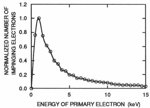
Fig. 5 The distributions of energy of multipactoring electrons at the transmission power of 4 MW
