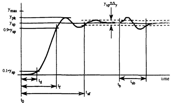
Figure 4. Response of the LLRF control to an RF signal.
