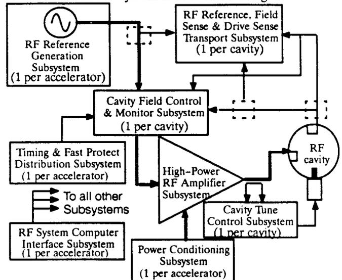
Figure 2. Simplified block diagram of a LINAC RF system
