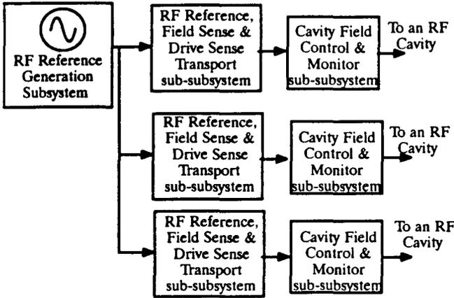
Figure 3. Star configuration of an RF generation/ distribution subsystem
