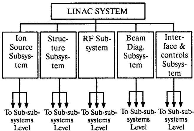
Figure 1. Simplified block diagram of the system configuration of a LINAC
