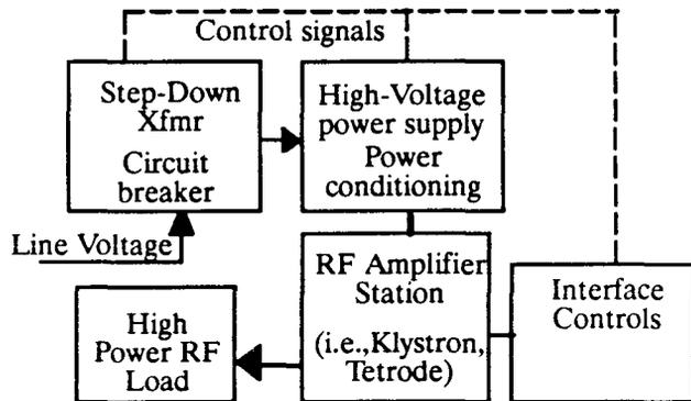
Figure 5. Block diagram of a HPRF subsystem
