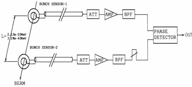
Fig.1 Block diagram of velocity monitor
