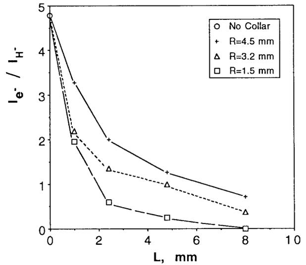
Fig. 4 The  $e^-$  to  $H^-$  current ratio  $I_{e^-}/I_{H^-}$  vs the collar length  $L$  for fixed collar radius  $R$ . The lines connect the data points.
