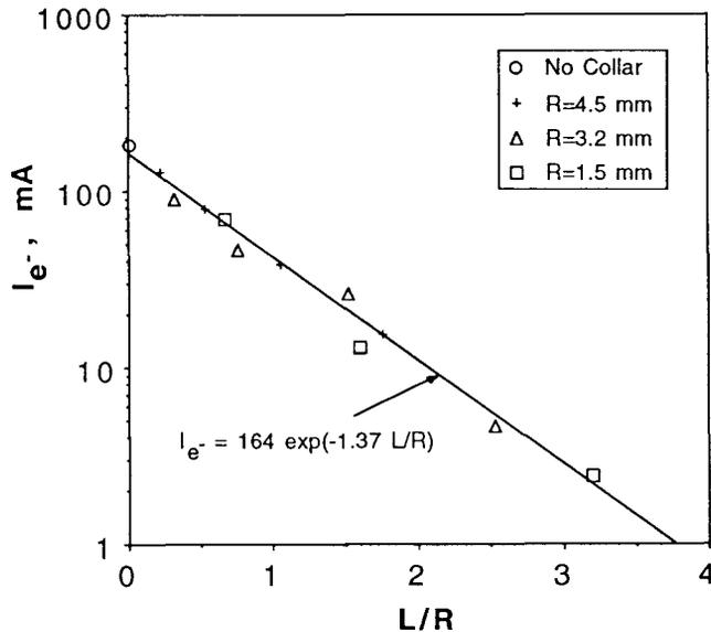
Fig. 6 A plot of  $I_{e^-}$  vs  $L/R$ , the ratio of the collar length  $L$  to the collar radius  $R$ . The line is a least-squares fit to the data.
