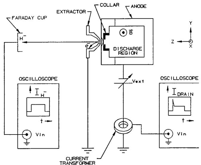
Fig. 2 Schematic of the  $H^-$  and  $e^-$  current measurements. The  $H^-$  current is measured directly with a Faraday cup. Because the  $e^-$  are deflected into the extractor electrode by the stray, transverse magnetic field, the  $e^-$  current is the difference between the drain current and the  $H^-$  current.
