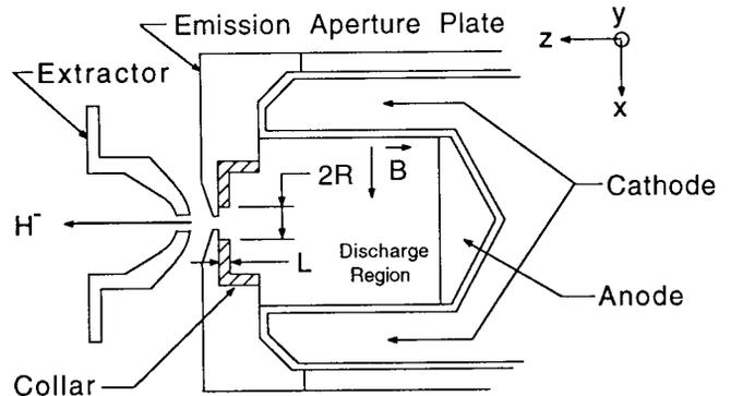
Fig. 1 The 8X-source collar geometry. The cylindrical collar insert (hatched area) is placed in the drift region between the emission aperture and the discharge region. The collar's length is  $L$  and its diameter is  $2R$ .
