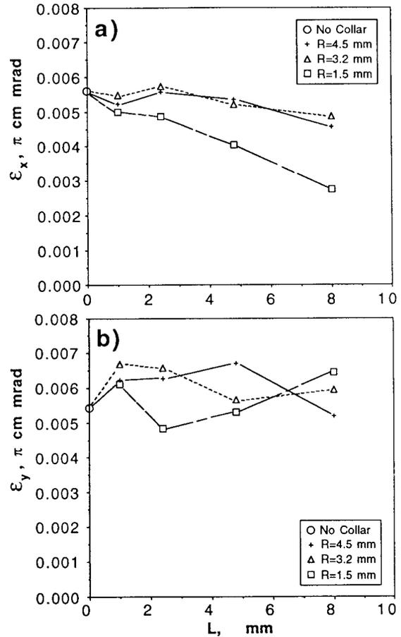
Fig. 5 a) The rms normalized emittance  $\epsilon_x$  vs the collar length  $L$  for fixed collar radius  $R$ . b) Same as a), except  $\epsilon_y$  vs  $L$ . The lines connect the data points.
