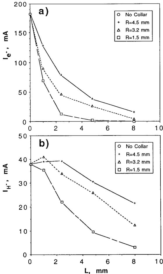
Fig. 3 a) The electron current  $I_{e^-}$  vs the collar length  $L$  for fixed collar radius  $R$ . The circle is  $I_{e^-}$  for no collar. b) The  $H^-$  current  $I_{H^-}$  vs the collar length  $L$  for fixed collar radius  $R$ . The circle is  $I_{H^-}$  for no collar. The lines connect the data points.
