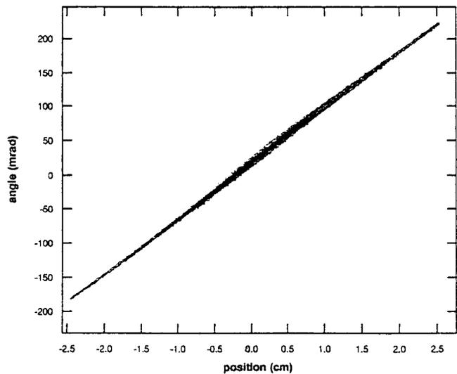
Fig. 4 Vertical  $H^-$  Phase-Space emittance plot
