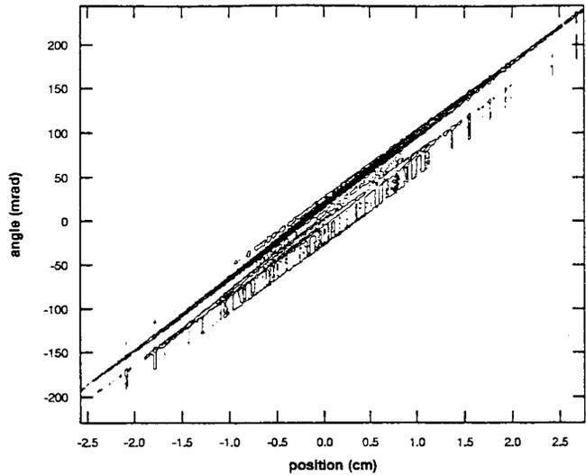
Fig. 3 Vertical Phase-Space emittance plot
