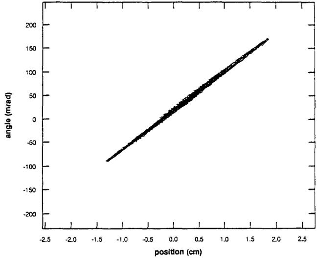
Fig. 6 Vertical  $\text{H}^-$  Phase-Space emittance plot with the wings cut off
