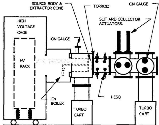
Figure 1. Magnetron Source test stand
