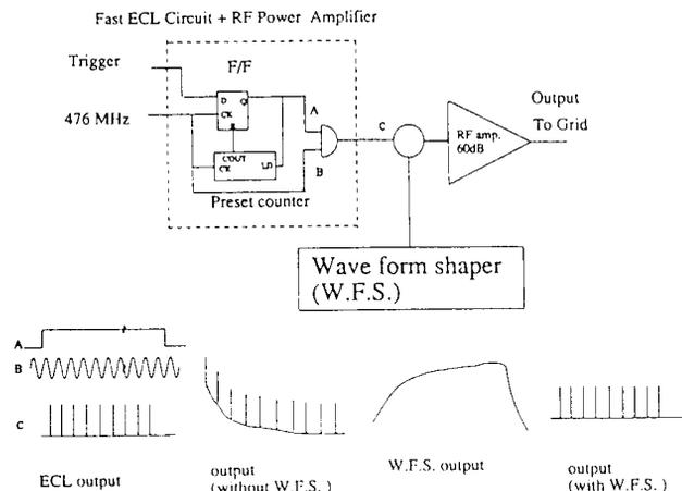
Fig 4 Schematic drawing of multi-pulse generator.
