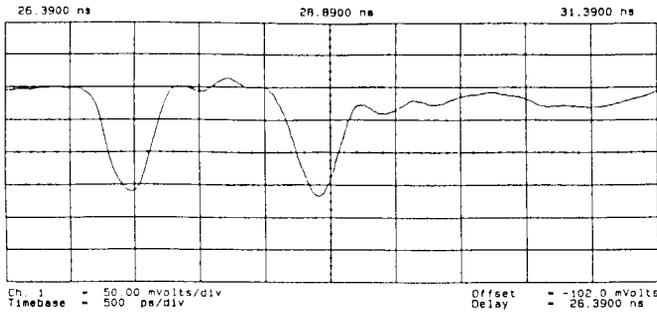
Fig.2 Output of the double-pulse generator (100V/div, 500ps/div)
