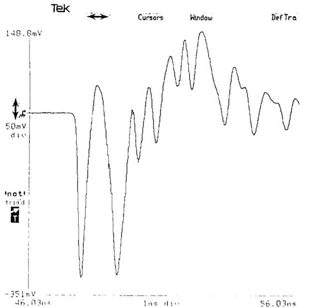
Fig 3 Wave shape of double bunches beam, Anode voltage: 170 kV, Heater voltage: 6.0 V, Net drive voltage: 260 V, Vacuum  $2 \times 10^{-8}$  Torr
