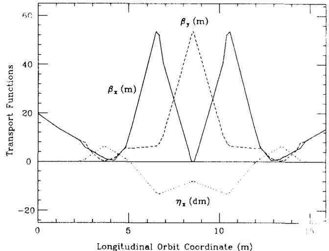
Fig. 2 NP beam parameters in the bypass transport.
