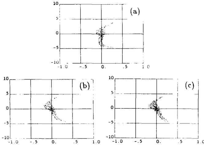
Fig. 3 NP bunch longitudinal phase space (keV vs. deg): (a) exiting the NP cryounit, (b) without bypass, entering the injector linac, (c) with bypass, entering the injector linac.
