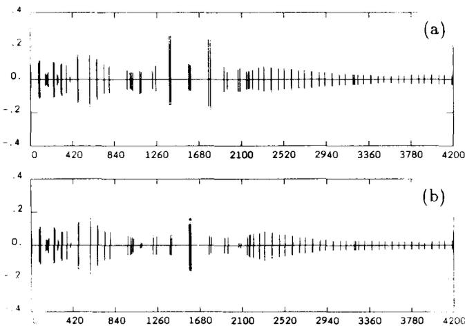
Fig. 4 NP beam envelope from the electron gun to the end of the injector linac, with the bypass transport (cm): (a) horizontal, (b) vertical.
