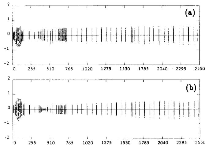
Fig. 5 High peak current beam envelope from the photoemission gun to the end of the injector linac (cm): (a) horizontal, (b) vertical.
