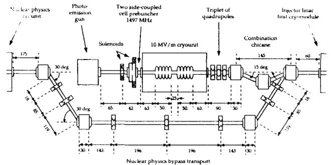
Fig. 1 High peak current source and NP bypass transport (dimensions in cm).
