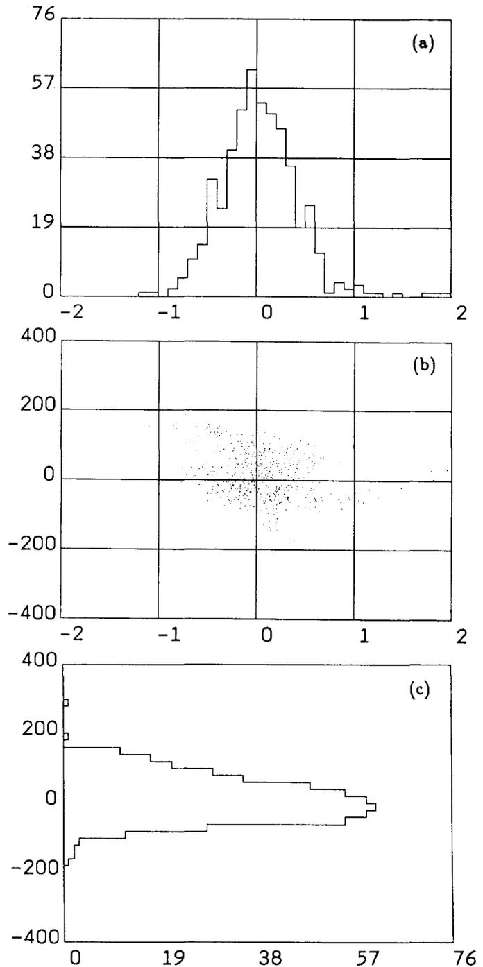
Fig. 6 Output of the high peak current source at the entrance to the injector linac: (a) phase spectrum (deg), (b) longitudinal phase space (keV vs. deg), (c) energy spectrum (keV).
