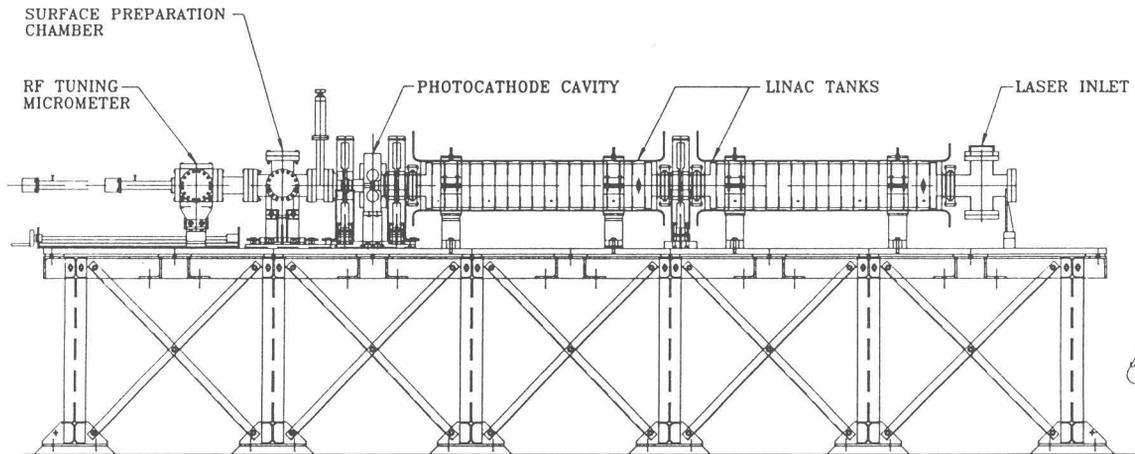
Figure 2. AWA photocathode gun and preaccelerator.
