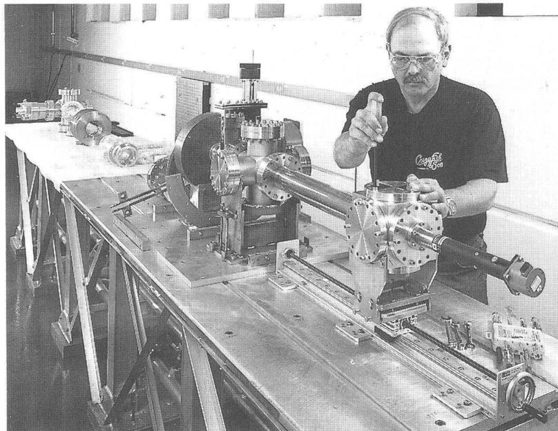
Figure 3. Photocathode and associated components.
