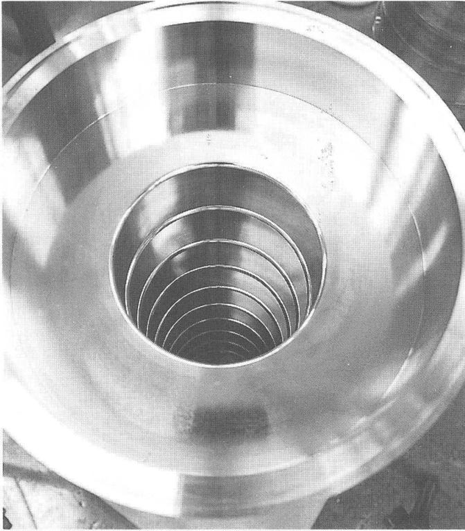
Figure 4. Linac cell stack.
