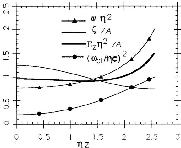
Fig 2 Electric field and other quantities (normalized) for  $B=0.25$  and  $R=2/3$ ; half a period is shown.
