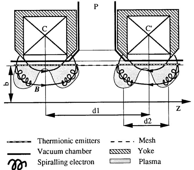
Fig 1 One cell CC' of the structure. P is the pump port.
