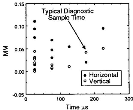
Fig. 6. Horizontal and vertical MM (IMS output beam) versus time within the macropulse. Maximum MMs are  $\sim 0.1$  in  $x$  and  $\sim 0.05$  in  $y$  indicating no significant changes in the CS parameters during the macropulse.
