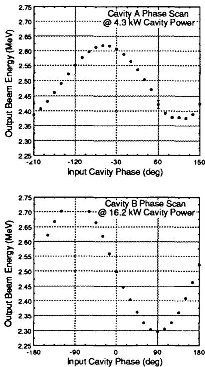
Fig. 2. Output beam energy as a function of the input cavity phase for the two IMS bunchers. Cavity A and B refer to the upstream and downstream cavities, respectively. For the data shown, the two cavities were operated at their design power levels. To operate the cavities in the bunch mode, the input cavity phase settings for cavities A and B are  $\sim -146$  and  $\sim -180$  deg, respectively.
