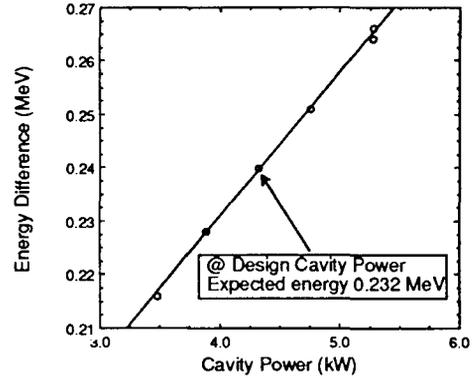
Fig. 3. Measured beam energy difference between the acceleration and deceleration modes for cavity A as a function of the rf cavity power. At the design cavity power, the expected and measured energy differences were 0.232 and 0.240 MeV, respectively.
