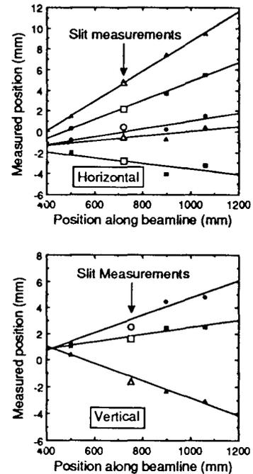
Fig. 1. Measured horizontal and vertical beam centroids along the beamline. Shown are data from the three D-plate microstrip probes and the emittance gear slit. Each line corresponds to a different steering configuration in the IMS.
