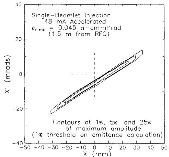
Fig. 2 RFQ1-1250 output emittance for single beamlet injection.
