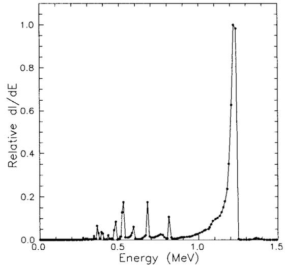
Fig. 4 RFQ1-1250 energy spectrum at 80% of design field.
