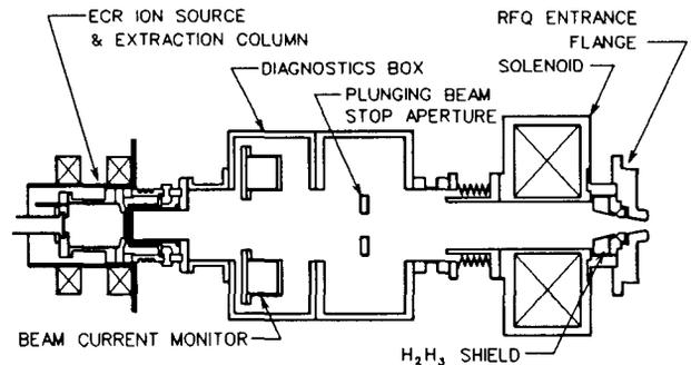
Fig. 1 Direct injection ECR ion source and LEBT.
