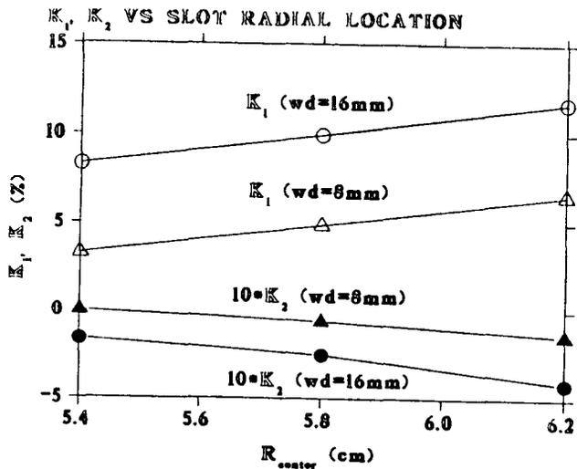
Figure 3:  $K_1$  and  $K_2$  vs slot radial location. Slot center angle=60°, width=8 and 16 mm. (MAFIA)
