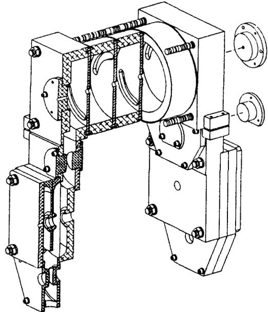
Figure 1: Geometry of the magnetically coupled bridge coupler
