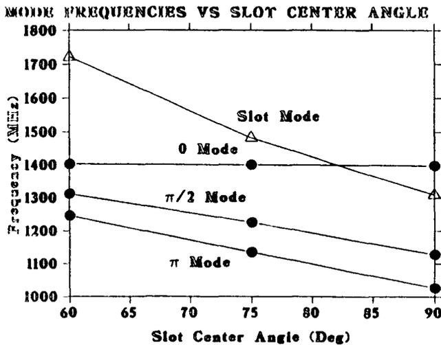
Figure 4: 0,  $\pi/2$  and  $\pi$  mode frequencies vs slot center angle. Slot width=16 mm,  $R_{center}=62$  mm. (MAFIA)
