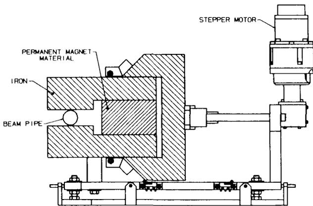
Figure 3: A schematic of the AFEL variable-field permanent-magnet dipole.
