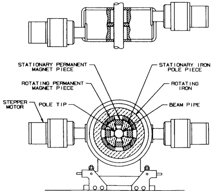
Figure 4: A schematic of the AFEL variable-field permanent-magnet quadrupole.
