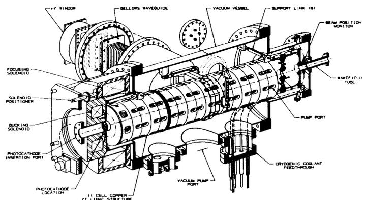
Figure 2: A schematic of the AFEL high-brightness linac.
