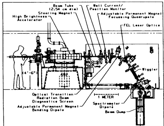
Figure 1: A schematic of the Advanced Free-Electron Laser System at Los Alamos.
