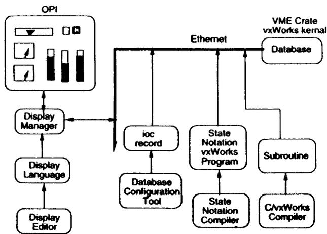
Figure 6: A schematic of the software environment of the AFEL computer-based control system.
