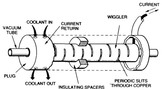
Figure 5: A schematic of a pulsed-current wiggler.
