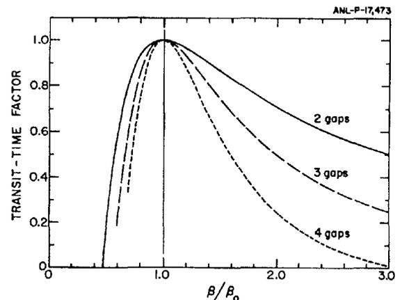
Fig. 1 Transit-time curves for accelerating structures.
