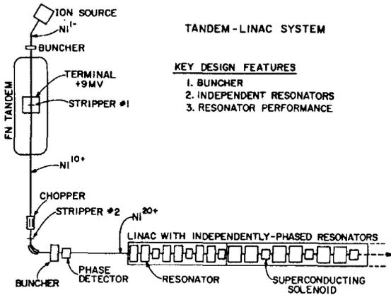
Fig. 2 Main components of a tandem-linac system.
