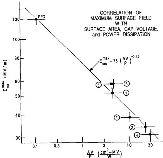
**Fig. 4** Dependence of  $E_{sur}^{max}$  on AV/P. The numbers attached to data points refer to the structures in Table 3.
