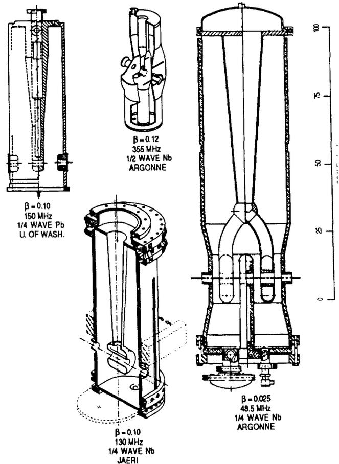
Fig. 3 Examples of recent accelerating structures.
