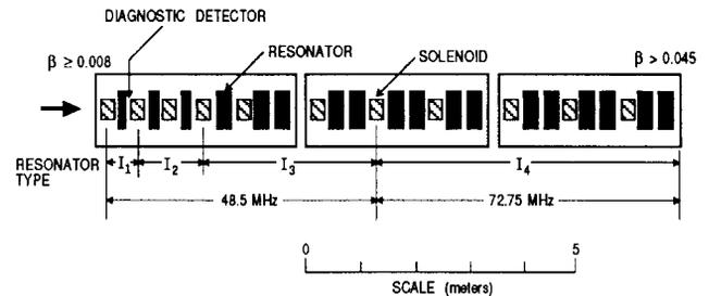
Fig. 6 Configuration of the injector linac of PII.
