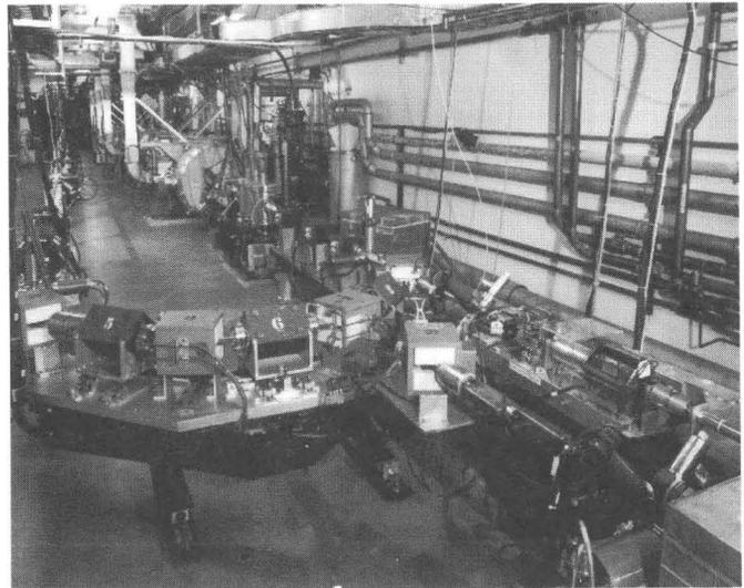
Figure 5. The first 180° bend of the recirculation system, mounted on a translation stage.
