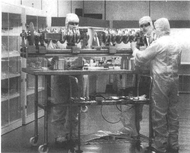
Figure 3. Clean room assembly of a CEBAF cavity pair.
