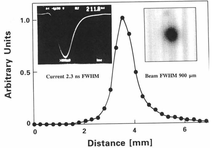
Fig. 8 Measured electron beam spot size in the interaction region.
