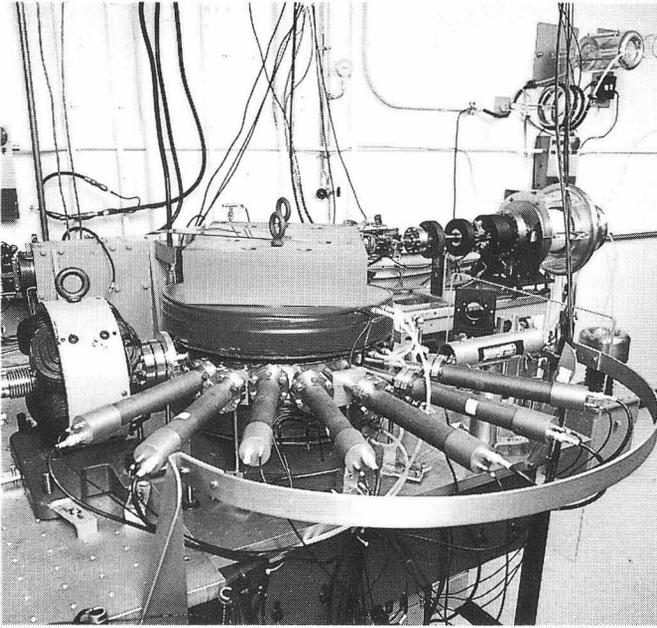
Fig. 6 Electron spectrometer and detector array.
