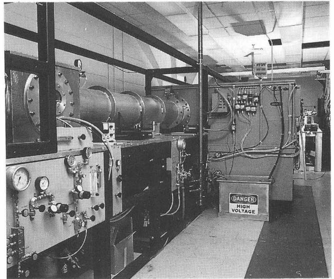
Fig. 3 The high-pressure CO<sub>2</sub> laser amplifier system.
