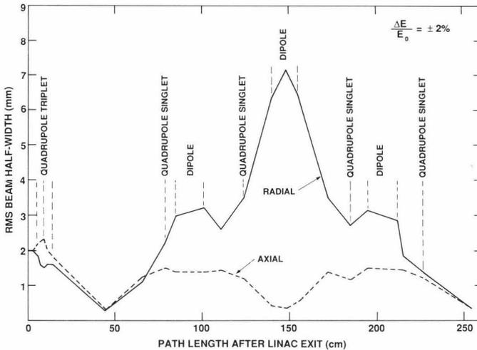
Fig. 7 Computer-calculated radial and axial beam profiles.
