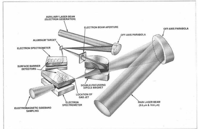
Fig. 9 Experimental arrangement to demonstrate acceleration of externally injected electrons.
