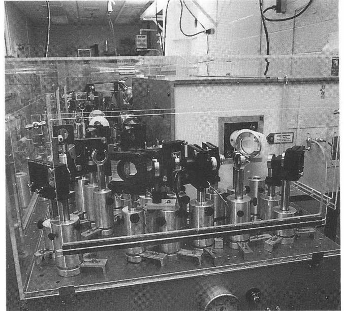
Fig. 2 The oscillator and the pre-amplifier sections of the CO<sub>2</sub> laser facility.
