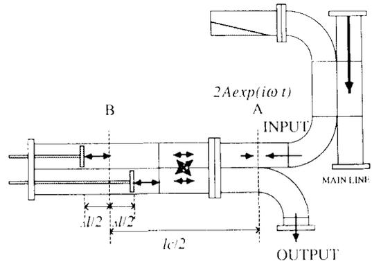
Fig. 1. Attenuator & phase-shifter for the prebuncher
