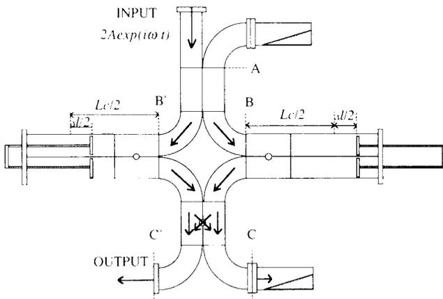
Fig. 2. Attenuator & phase-shifter for the buncher
