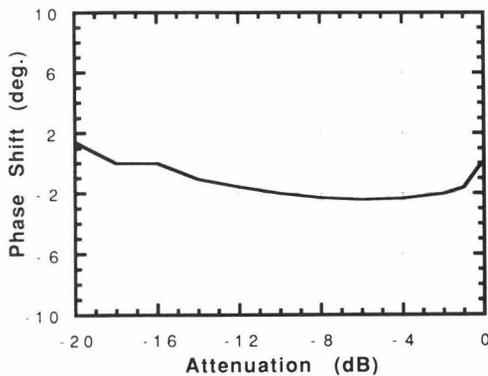
Fig. 5. Phase shift vs. attenuation at 2856 MHz
