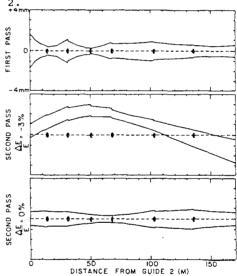
Fig. 2: Computer Simulation of beam envelope using the strong focussing solution for optimizing the energy band pass. The upper trace represents the first pass beam envelope. The lower traces represent the second pass on-energy beam and a beam off-energy by 3%.
