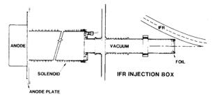
Schematic diagram of the new beam transport Fig. 13. and injection hardware.
