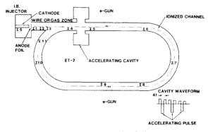
Fig. 1. Schematic diagram of the RLA.
