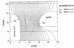
Fig. 4. Both the anode and cathode surface shapes are optimized for minimum electric field stresses.
