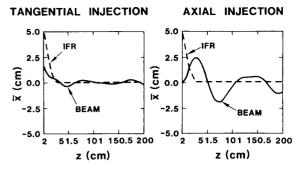
Fig. 12. Numerical simulation of beam injection obtained with the code BUCKSHOT. It appears that axial injection along the straight section of the racetrack IFR channel is not the right approach. The required injection angle and offset are functions of the beam energy and channel charge neutralization factor f.
