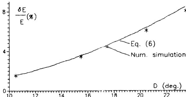
Fig.4 The value of the RF amplitude underestimation vs the root-mean-square bunch size D (  $D\varphi = D\beta \cdot w/\Omega = D/2$  ).
