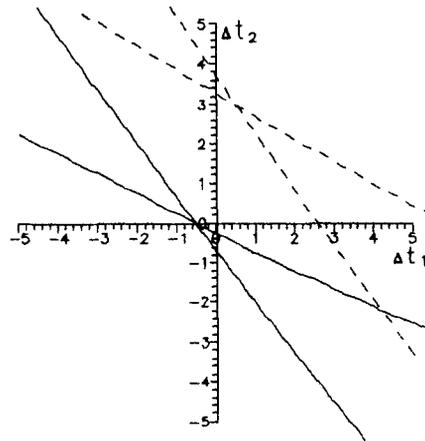
Fig.2 Curves of the phase scanning for the first cavity of MMF linac before (dashed lines) and after (solid lines) correction of "nonideality" of the cavity.
