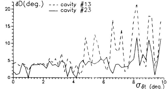
Fig.5 The error of the bunch size vs the dispersion of the normal random error of the  $\Delta t$ -measurements.
