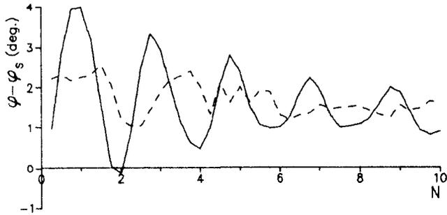
Fig.3 Phase oscillations of the bunch center vs cavity number for various input phases. Simulation has been made without instabilities of the accelerating field.
