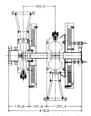
Scale drawing of the rf-driven lasertron Fig.5. (dimensions in millimeters).
