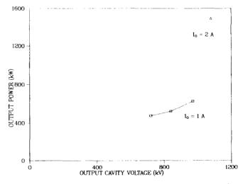
Fig. 2. Calculated output power versus output cavity voltage for the system of Fig. 1, with average beam current as the parameter.
