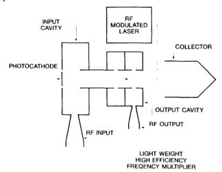
Fig. 1. Schematic drawing of the rf-driven lasertron experiment.
