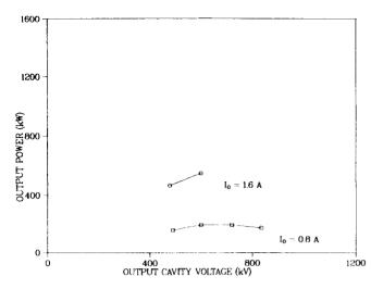
Calculated output power versus output cavity Fig. 3. voltage for the five times lasertron frequency multiplier, with average beam current as the parameter.
